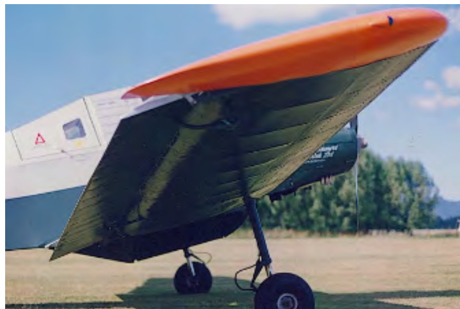
UPPER: Barbara Hope-Cross seen beside ZK-BXO in the early 1990s, lending scale to the aircraft. LEFT: Underside details showing undercarriage, ailerons and top-dressing hoppers.
