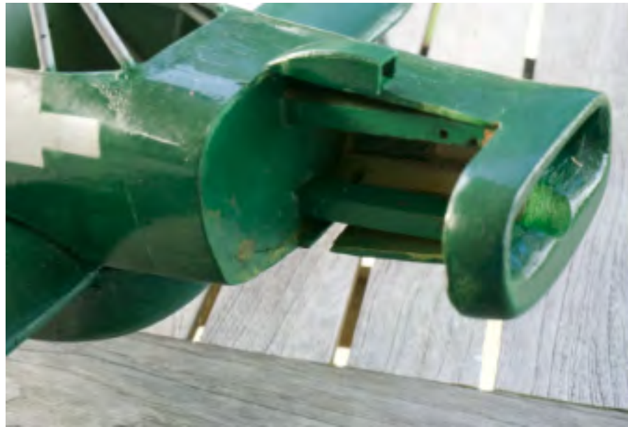
RIGHT: The cowling layout has been revisited and shows plenty of room for the side-mounted engine and tank. .
