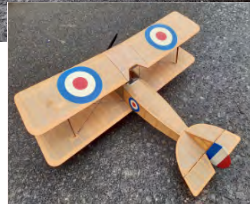
ABOVE: The Sopwith Tabloid now re-engined with an outrunner electric motor and prop-saver.
